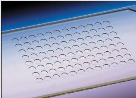
Micro titer plates are a growing market in biotechnology. The parallel investigation of small volumes speeds up the analysis. This micro titer plate is made of a polycarbonate sheet on glass. The wells have a diameter of 1,2 mm and a depth of 250  $\mu\text{m}$ .
